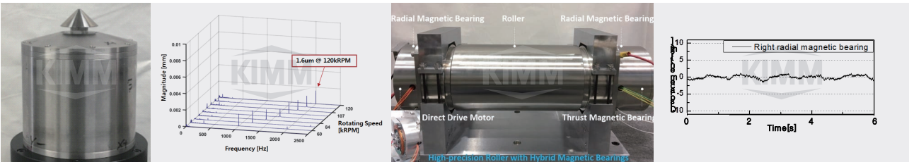
High-speed spindle with rotational speed of 120,000 rpm
