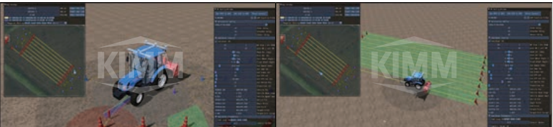
〈3D-Based Tractor Unmanned Operation Virtual Test and Work Path Visualization Technology〉
