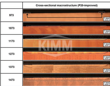
◁ Example of Heat Treatment Technology of Metallic Material Using Large-area Diode Laser for Mold Steel Application ▷
