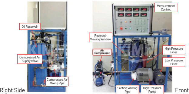
◁ Image of Prototype of Oil Reservoir with Tilted Return Line ▷
