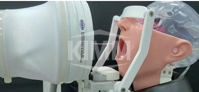
〈 Non-Face-to-Face Remote Specimen Collecting Robot System〉
