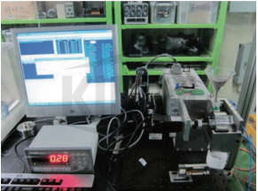
〈 Dispensing Performance Evaluation and Powder Control Test Device Using Metal Powder 〉
