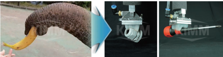
〈 Just like the movement of the tip of the trunk of an elephant, it can hold an object by covering the outer shape of it 〉
