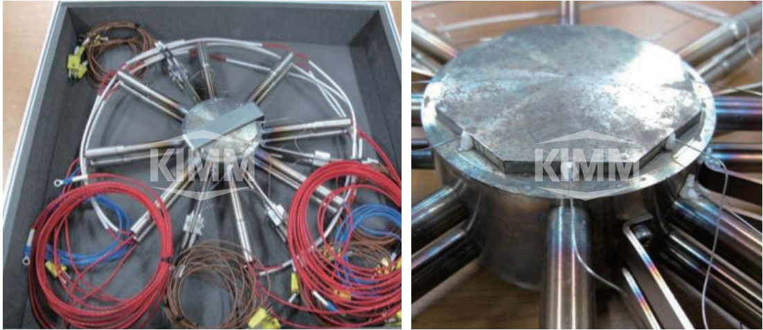
〈 2D Heat Flux Gauge Block : Heat Flux Measuring Apparatus 〉
