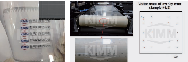
◀ Mesh Type Transparent Electrode Using Reverse Offset Printing ▶ ▶ Roll-to-Roll Reverse Offset-Printed Registration Print Sample and Registration Accuracy Measurement Result (Registration error vector map)
