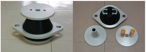
Hybrid Mount for 100 kg Class (serial, rubber mount + piezoelectric actuator) A study on the hybrid mount against vibration and shock for naval ships, J. Shock and Vibration, 2010
