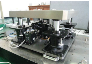
Hybrid Mount System (serial, air spring + piezoelectric actuator) Feasibility study on a hybrid mount system with air springs and piezostack actuators for microvibration control, J. of Intelligent Material System and Structures, 2012
