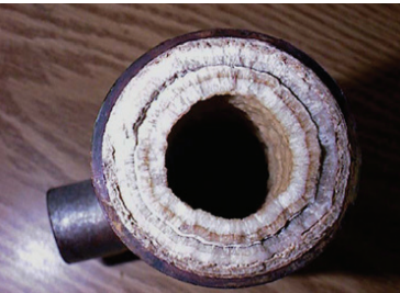
Existing Pipe Scale and Newly Developed and Installed Scale Removal Device
