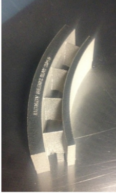
Photo: Nozzle-guide vane segment for jet engine made of IN718
