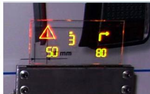
emissive HUD with integrated diodes
