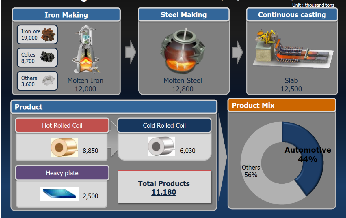
Figure 21. Manufacturing Process & Product Mix (Integrated Steel Mill)
