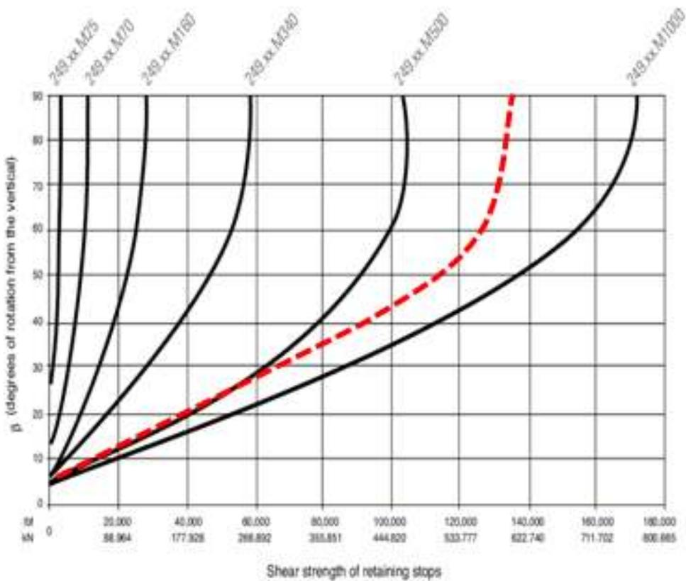
[ $\beta$ (degrees of rotation from the vertical) – Shear strength of retaining stops 선도]
