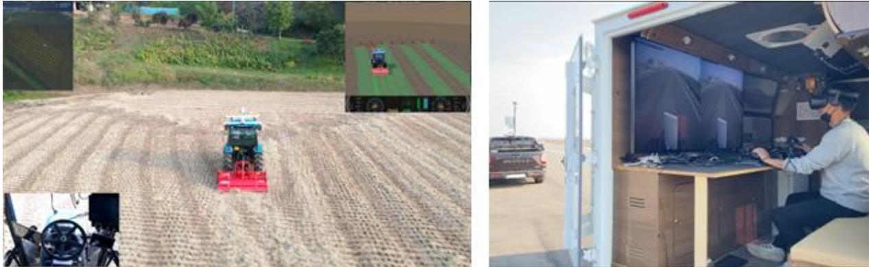
Photo description: Unmanned tractor at work using KIMM's VR-based unmanned working vehicle virtual test and control technology (left), and remote operation by a user wearing a head-mounted display (HMD). With KIMM's VR-based unmanned working vehicle virtual test and control technology, unmanned operations can be performed using pre-designed algorithms, and effective integrated control is enabled through real-time monitoring of results.
