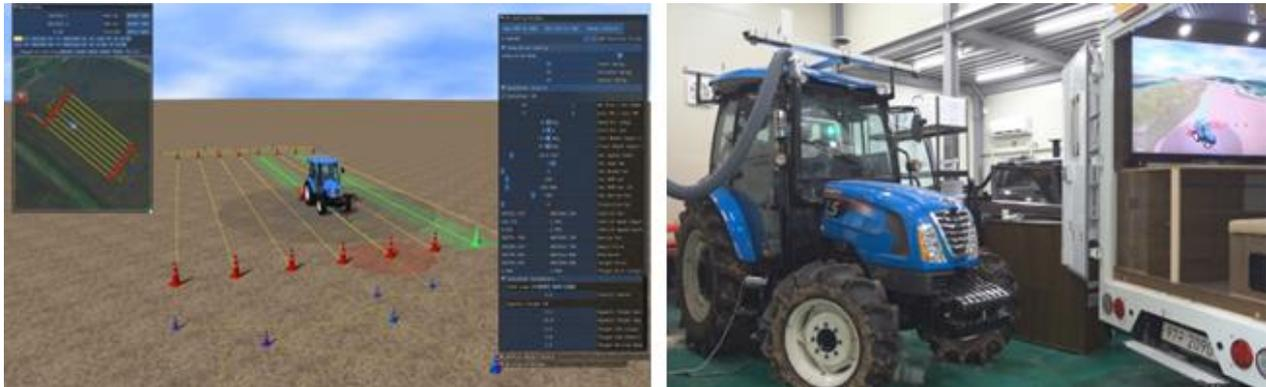
Photo description: The virtual test software for unmanned working vehicles developed by KIMM (left) and virtual testing using an actual unmanned tractor (right). With KIMM's VR-based unmanned working vehicle virtual test and control technology, unmanned vehicles can be tested on various paths and under different scenarios before real-world operation.
