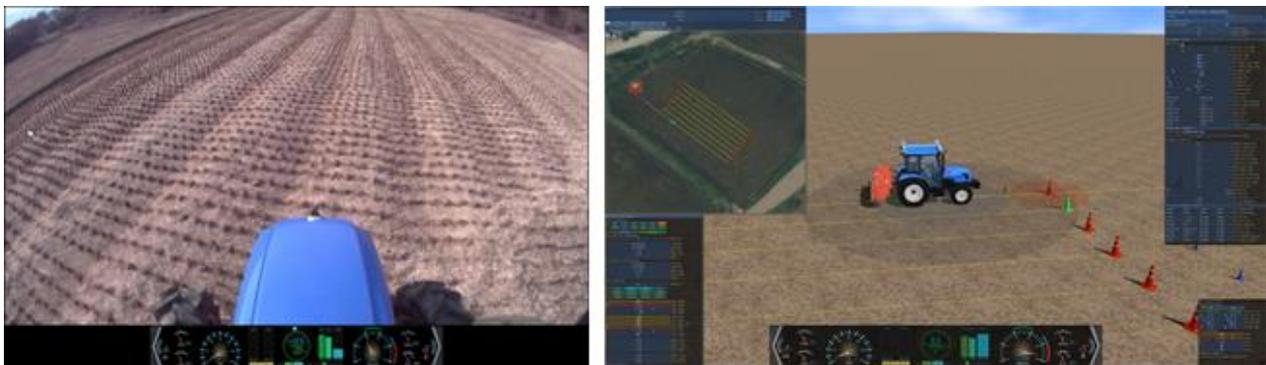
Photo description: Remote video control using KIMM's VR-based unmanned working vehicle virtual test and control technology (left), and monitoring of task execution by the tractor in the 3D software (right). With KIMM's VR-based unmanned working vehicle virtual test and control technology, the user can perform virtual tests to determine whether the machine works as desired in outdoor environments.
