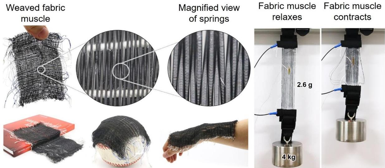
Photo description: Fabric muscle developed by the research team led by Dr. Cheol-Hoon Park of KIMM. Shape-memory-alloy springs were weaved in the same method as fabric, and the resulting light and soft fabric muscle is capable of carrying up to 1,500 times of its own weight.
