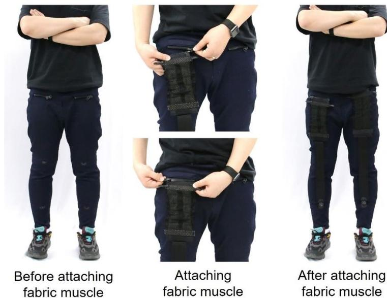
Photo description: The fabric muscle developed by Dr. Cheol-Hoon Park’s team transforms regular pants into a suit-type wearable robot. The fabric muscle can be attached to desired body parts for use as “wearable muscles.”
