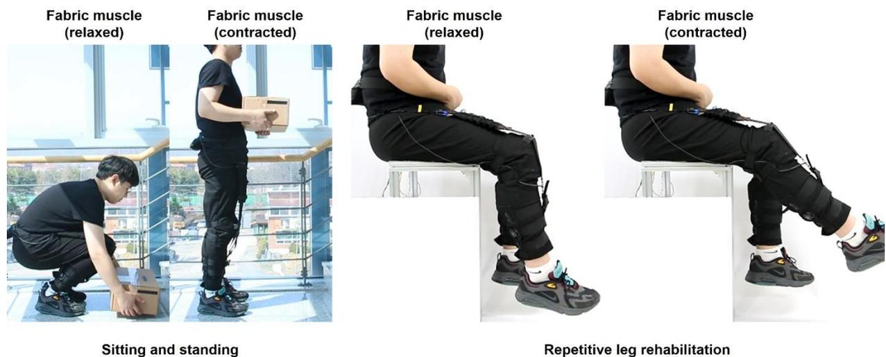
Photo description: Applications of the fabric muscle developed by Dr. Cheol-Hoon Park’s team. The fabric muscle can be used to assist wearers in sitting and standing, climbing stairs, and rehabilitation training involving repetitive movement of arms and legs.
