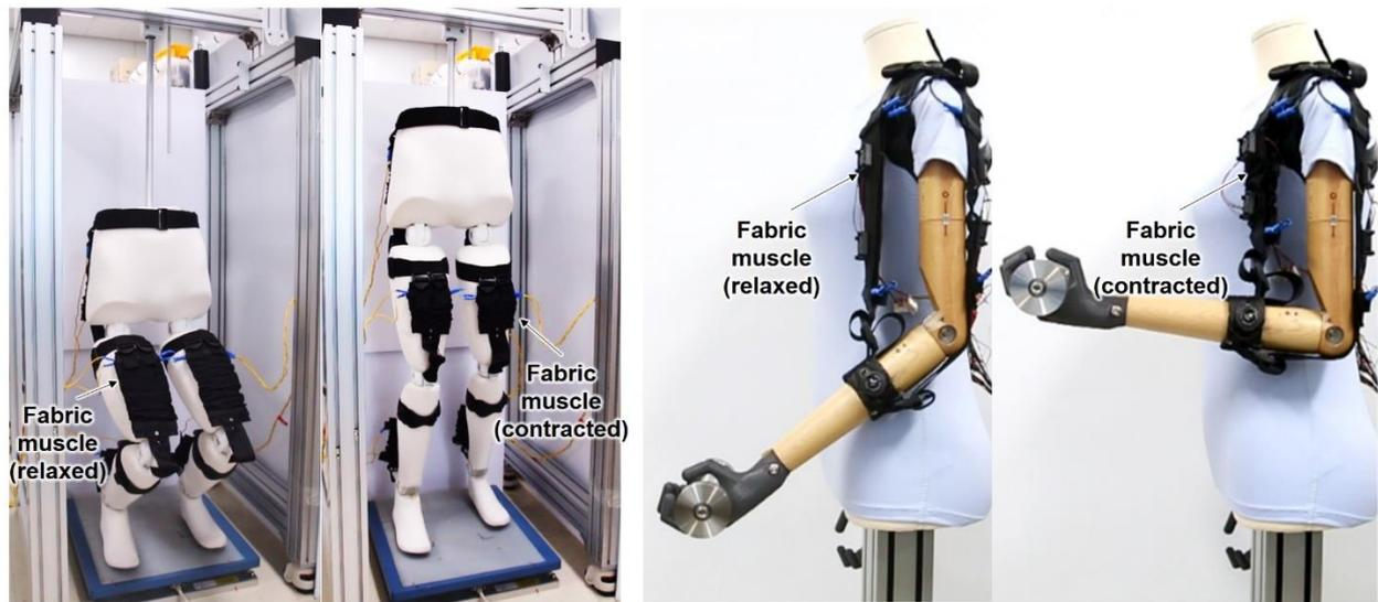
Photo description: Dr. Cheol-Hoon Park's team gives a demonstration of the fabric muscle providing strength assistance to a mannequin. The force generated by the fabric muscle allows the mannequin to stand (left) and carry heavy objects (right). Similarly, the fabric muscle can be attached to body parts requiring strength assistance.
