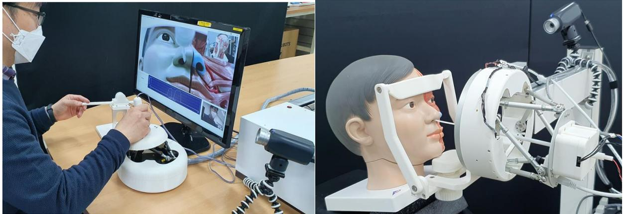
Photo description: The KIMM research team led by Dr. Joonho Seo is performing a demonstration of the non-face-to-face remote sampling robot. When the operator moves the master device, the slave robot at the remote site retrieves a sample according to the operator's movement.
