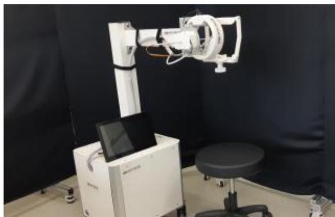
Photo description: Slave robot of the non-face-to-face sampling system developed by Dr. Joonho Seo of KIMM
