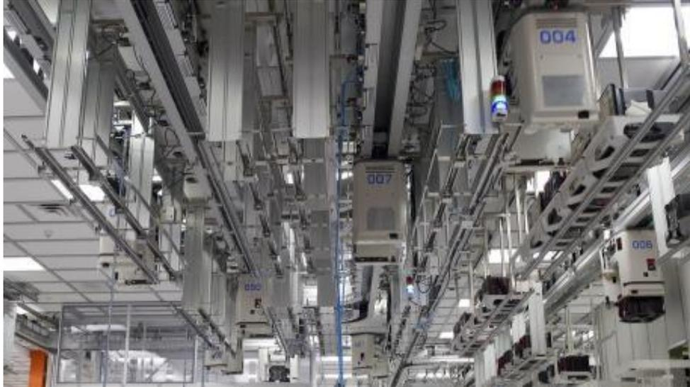
Photo description: The photo of newly developed 2D LiDAR sensors for semiconductor wafer transfer equipment. This photo shows the semiconductor wafer transfer equipment (OHT) with 2 to 4 LiDAR sensors attached to each equipment.
