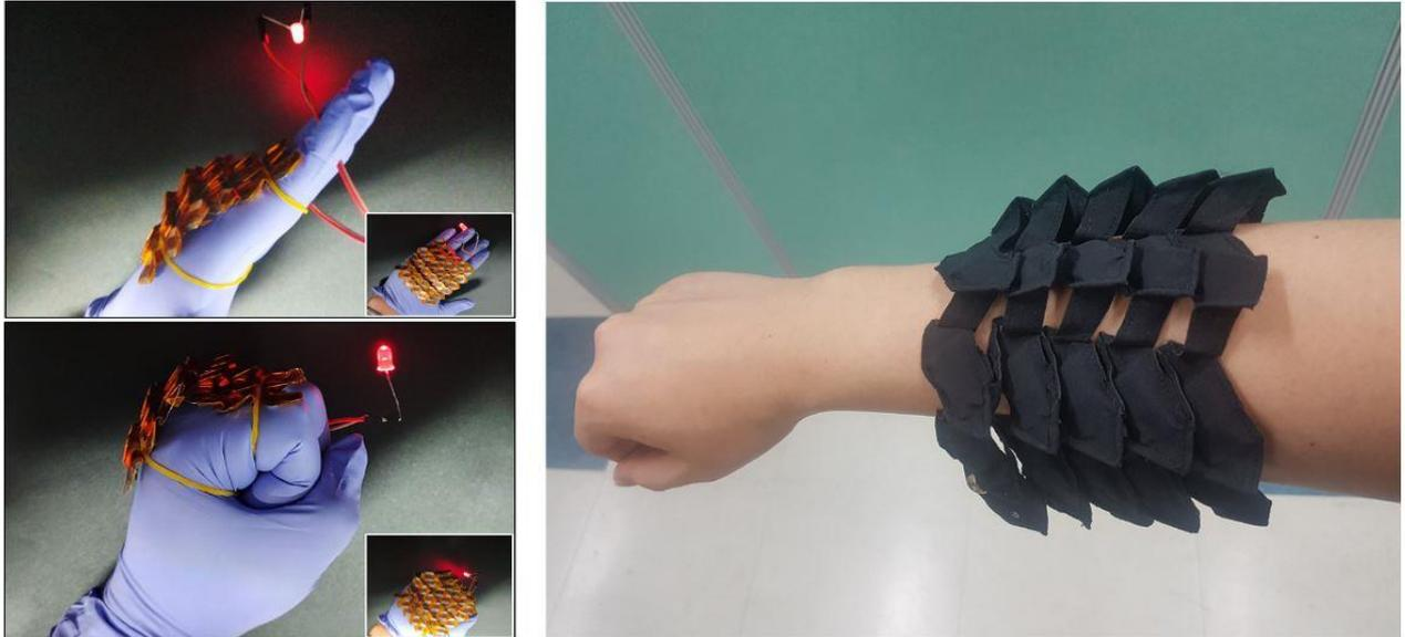
Description: The flexible, stretchable battery developed by the research team of Dr. Bongkyun Jang and Seungmin Hyun at the KIMM Department of Nano-Mechanics is shown on an individual's arm and hand. The battery is not only capable of conformably attaching to the shape of the human body, but can also morph freely to match the wearer's movement.
