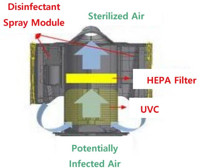
Description: Conceptual diagram of the robot system and the installed infectious disease prevention module to perform autonomous infectious disease prevention tasks.
