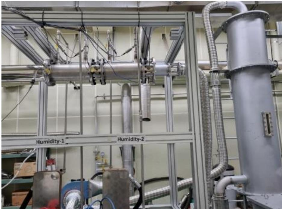
Description: Principal Researcher Dr. Youngmin Kim of the Department of Engine Research at the KIMM has developed a hybrid cooling and absorption condensable particulate matter removal technology that can simultaneously remove white smoke and condensable particulate matter. This technology removes exhaust gas generated from a boiler installed in the laboratory through a primary cooling and secondary absorbent method.
