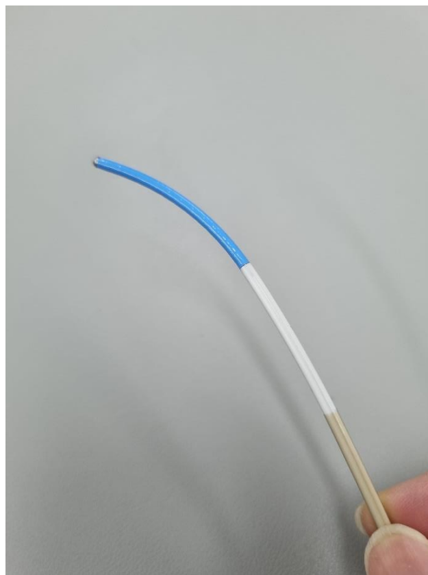
Description: A photo of robotic catheter distal bending site. This is an inner guiding catheter with a diameter of 2.8 mm.
