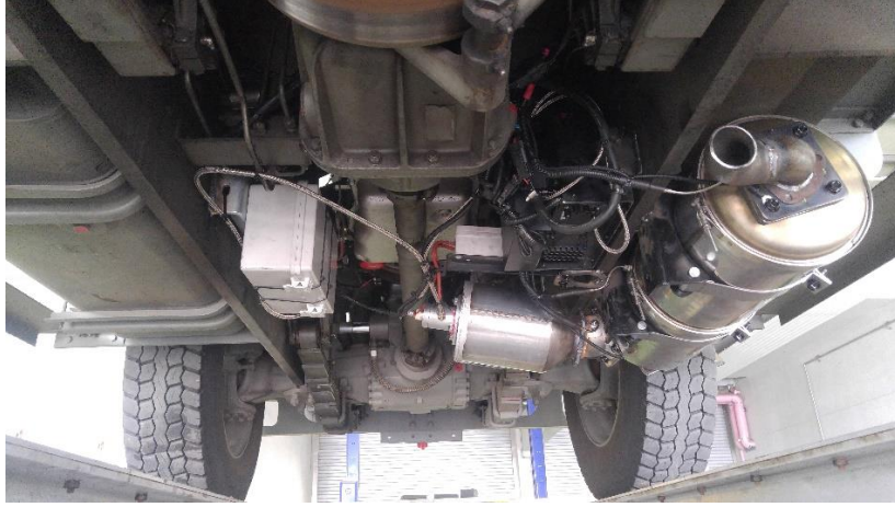
Description: A photo of Plasma DPF System installed in a special Korean military vehicle.
