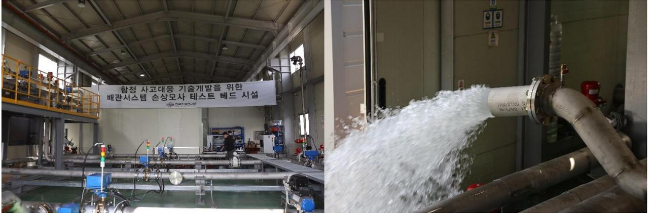
Description: (Left) Test Bed for Rupture Tests (downsized firemain of a Naval Ship): Ten K-smart valves are installed at each zone. If a pipe in any zone is ruptured, closely located valves are autonomously closed to isolate the rupture.
