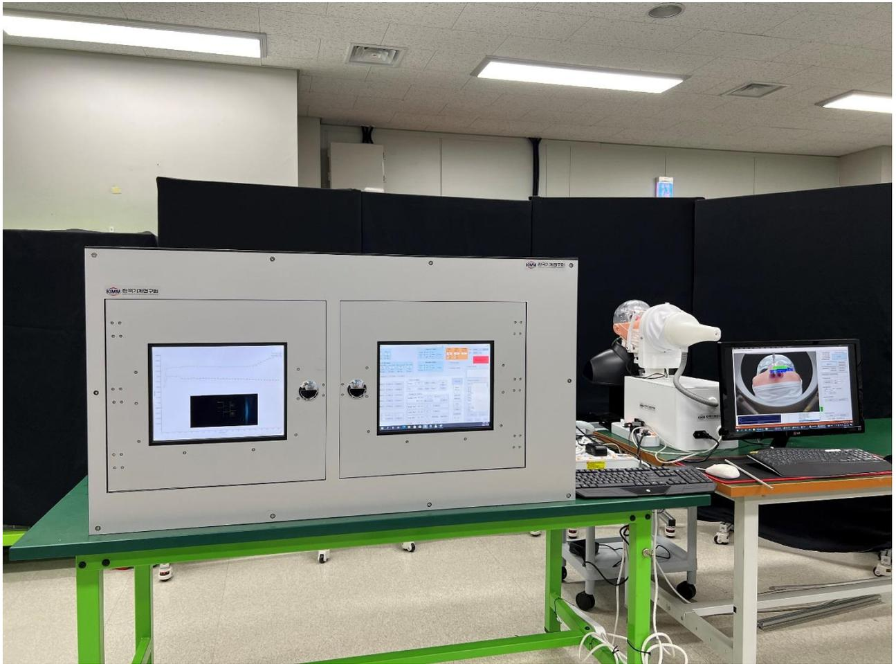
Description: A photo of the rapid, automated molecular diagnosis system integrated with a sample collection robot.
