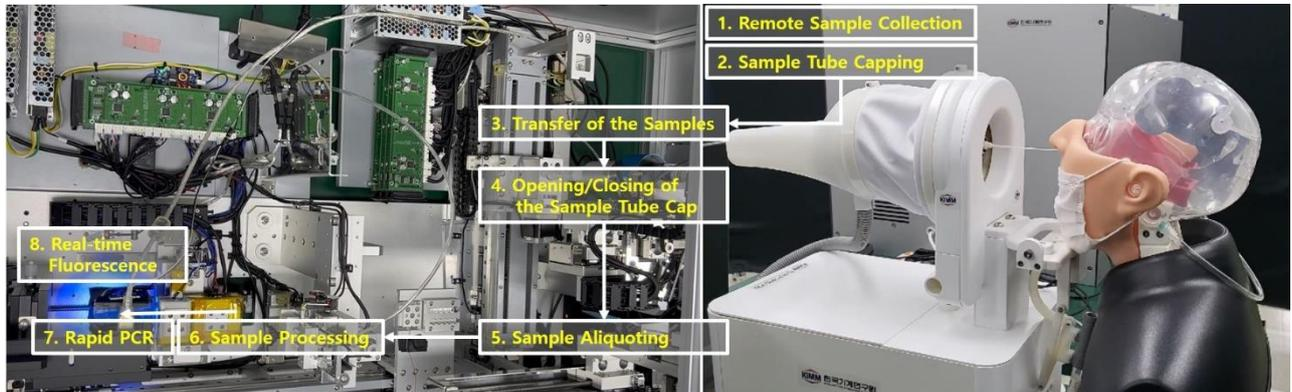
Description: Operation procedure of the rapid, automated molecular diagnosis system with a sample collection robot.
