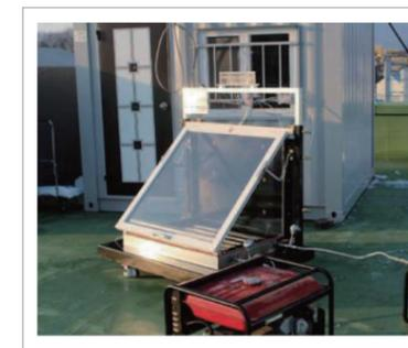
the fresh water production ability of solar still with verified durability and the multiple-effect technology that can boost the efficiency.
