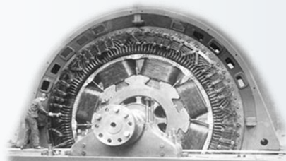
Siemens single-phase generator
