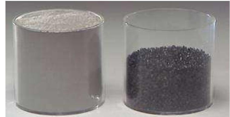
Flyash (Conventional Boiler) Grassy Molten Slag (IGCC)
