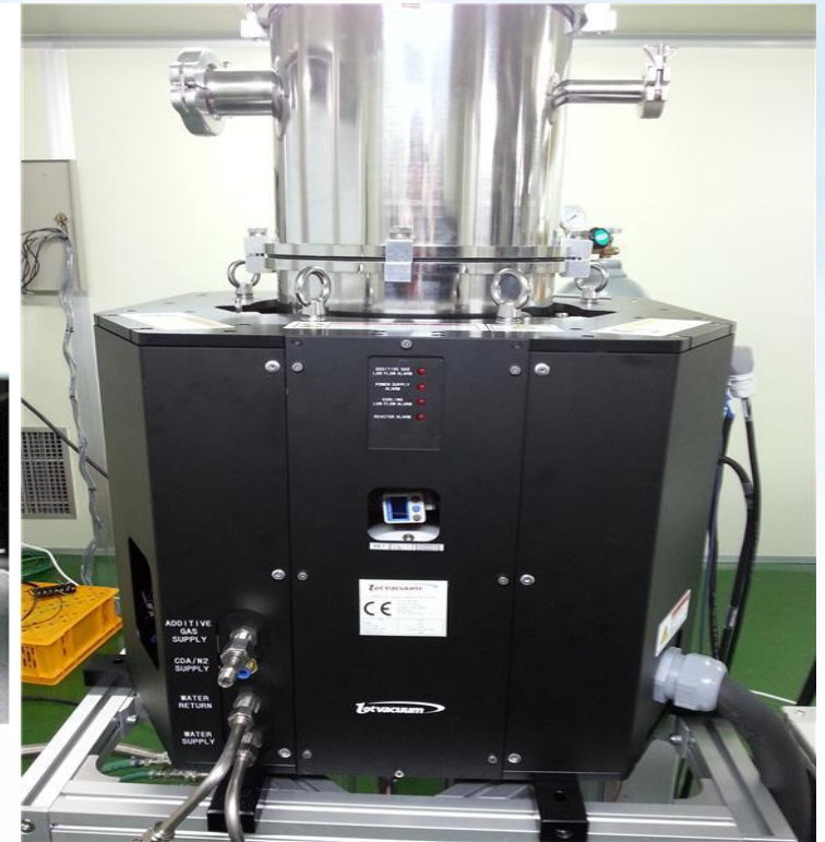
Plasma reactor for abatement of PFCs gases emitted from the semiconductor manufacturing process
