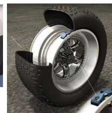
Tire pressure sensor
