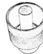
d) Planetary gear: diff. preforms (thin-walled tripple-cup) and finished part filled with CFRP
