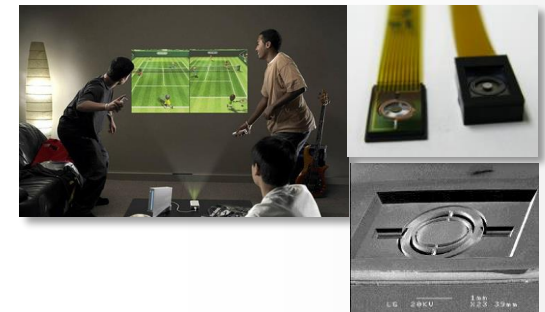
Laser Scanner for Pico Projector ('06~)
