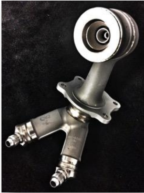
GE fuel nozzle: 19 individual parts combined into one
