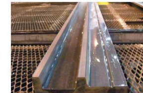
Rail production by roll-forming process
